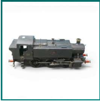
5-inch gauge live steam model of a GWR 15XX 0-6-0 Pannier Tank locomotive
